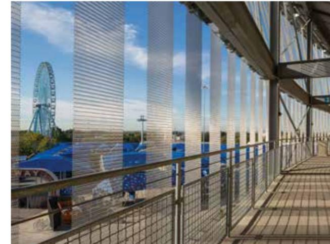
*We used two different scales of mesh, which became a design tool. We placed long ribbons of smaller scale stainless mesh from the top of the structure all the way down to the bottom. Then, on the upper portion of the structure, we used the larger scale stainless mesh that reflects much more sunlight. When we overlap the two, you sense the depth between both patterns as it transforms the surface into a diaphanous veil.*
